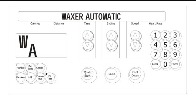
Upon entry into this test the letters WA (waxer automatic) will be in the profile window. This test allows the user to see information concerning the waxer motor. The waxer information will scroll automatically every 3 seconds.
